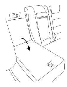
**WARNING:** Before returning the seatback to its original position, make sure that cargo or any objects are not trapped behind the seatback. After returning the seatback to its original position, pull on the seatback to ensure that it has fully latched. An unlatched seat may become dangerous in the event of a sudden stop or collision.
